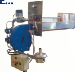
If you need to increase the process air temperature through a duct, by fixing the burner with a flange on the outside of the duct, this burner can be inserted inside the channel. It comes complete with combustion air blower and electrical panel to control and power the burner. Heating capacity from 70 kW to 756 kW.
