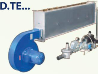
Burners for vertical dryers, similar to the VD series. However, the combustion body modules have a smaller surface area to ensure a reduction in heat capacity and good heat distribution throughout the air channel of the dryer. Heating capacity from 174 kW to 1750 kW.
