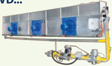
Traditional gas burners for direct fire in vertical dryers. With this type of combustion, the process air for drying, generated by the dryers fans, the combustion air generated by the burners fans and the combustion fumes, all mix together to form the air necessary to dry the product, reducing energy consumption. Heat capacity from 814 kW to 8150 kW.
