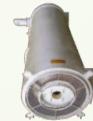
This regards combustion chambers designed and manufactured in steel by our sister company, Tecnecoforni Srl. These chambers are for indirect fire, where the combustion fumes, as opposed to the previous series, are expelled into the atmosphere and do not come into contact with the product to be dried. Heating capacity from 580 kW to 6000 kW.
