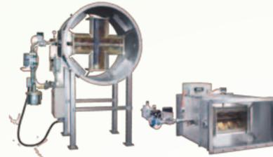
The burners of this series can have the same duct shape and combustion body configuration as the previous series. The only difference is that they use the process air from the plant for combustion. Heating capacity from 175 kW to 4300 kW.
